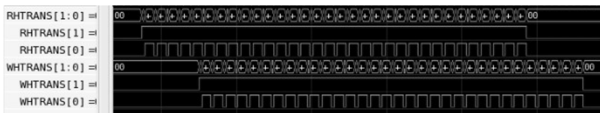
Illustration 12: Bus activity, single channel, 32 bit, buffer size 32 bytes, read and write outstanding
